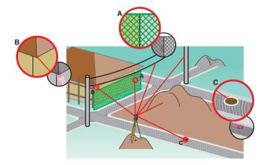
The ultra-narrow laser beam can measure precisely walls, corners, manholes on the road surface even chain-link fences and tree branches
