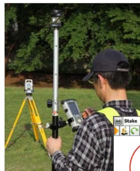
The DX series Auto Tracking Feature also brings advantages for one-man stake-out survey. Simply by moving the data collector, you'll be able to find the stake-out points easily and quickly, thus ensuring high productivity and accuracy for your stake out jobs. The difference in productivity can be clearly seen in the chart below.
