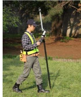
Auto tracking function the DX series of improves workflow of one-person TOPO survey drastically. You just hold prism pole and data collector and make swift, uncomplicated survey on numerous points; the steps necessary to complete the job are decreased by more than 30 percent as illustrated below.
